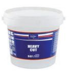
S07 polishing paste of the highest cutting level can be used on a mold or products made of industry gelcoat. It removes the deepest defects made during grinding with P800 paper. The paste does not contain silicone or wax fillers.
