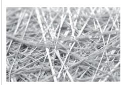
Glass fibre mat, in connection with laminating resin, is used for the repairs of big holes in boats, yachts, camping caravans, etc. The repaired elements may be made from steel, aluminum or GRP, reinforced with glass fibre. The obtained layers have very good adherence, are durable, resistant to petrol, oils, greases, and the short period temperatures up to 70°C.
